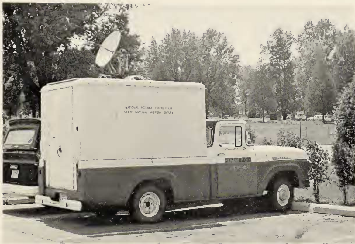
FIG. 1. Mobile radar unit used to observe bird migration at several localities in Illinois.
